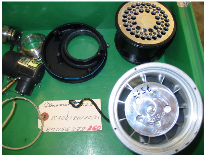
Figure 9: Turbine type gas flowmeter dismantled before inspection and recalibration at the manufacturer (Elster)
